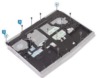
**3** Remove the two screws (M2x3) that secure the tron-light holder to the palm-rest assembly.
