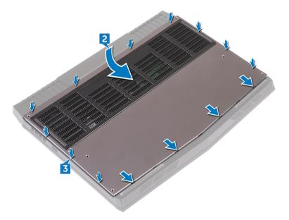
4 Tighten the captive screw that secures the base cover to the computer base.
