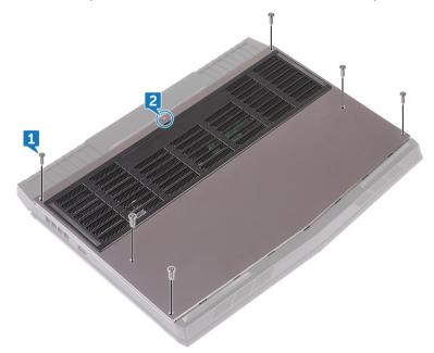
3 Using a plastic scribe, gently pry the base cover from the gap around the captive screw to release the clips on the base cover from the computer base.
